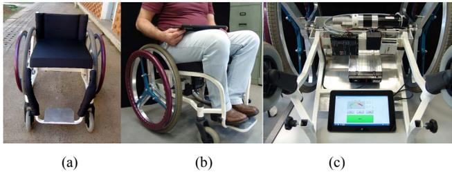
Fig. 2. Servo-assisted wheelchair prototype: (a) front view; (b) perspective view; (c) mechanical and electronic components under the seat.
