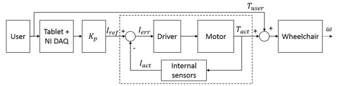
Fig. 3. Block diagram for the wheelchair control system
