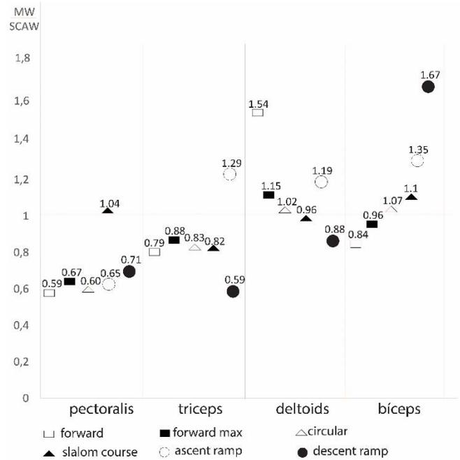
Fig. 6. Ratio (MW/SCAW) of the mean EMG for the manual wheelchair (MW) and servo-controlled assisted wheelchair (SCAW).
